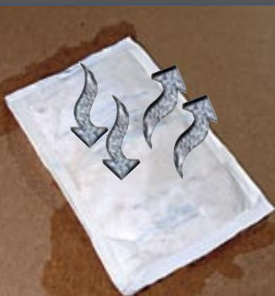
Due to the pouch design, the desiccant is immediately over-exposed and moisture protection quickly declines. And daily temperature fluctuations always cause a re-release (re-evaporation) of absorbed moisture back into the air. At high levels of humidity, the pouch type desiccant also easily becomes over-saturated and usually leaks.
