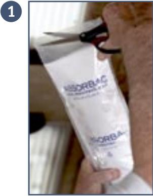
To remove the Absorbag Compact from its outer protective sleeve, cut open the sleeve at the top, making sure not to cut into the Absorbag Compact.
