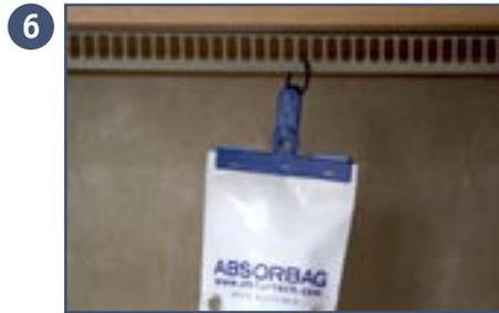
Now hang the Absorbag Compact by its hook in the cable tie. Note: Absorbag Compact works best if there is air circulation around the entire unit.
