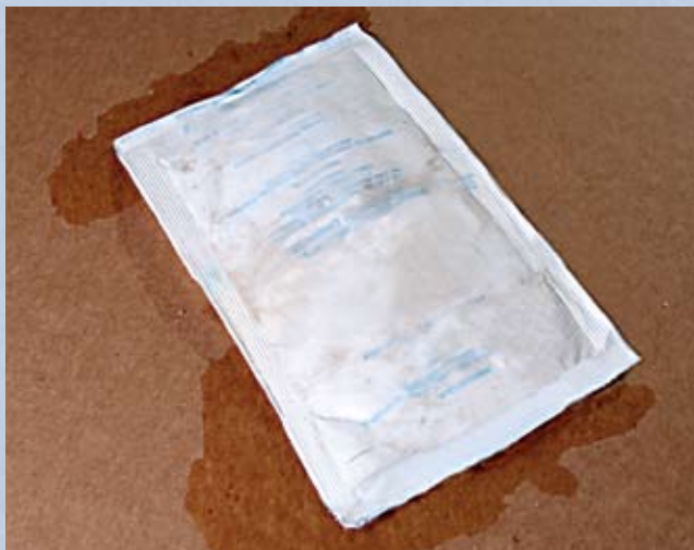
When the desiccant is needed the most—at high humidity levels—the pouch type easily gets over-saturated and stops absorbing. Once they become over-saturated, leakage also usually occurs.
